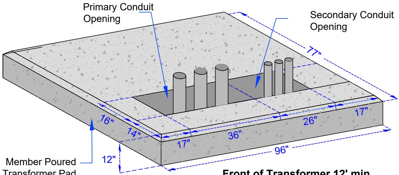
**Front of Transformer 12' min. clearance from any obstructions**
