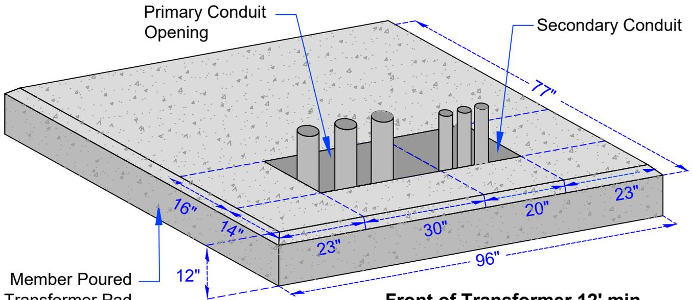
**Front of Transformer 12' min. clearance from any obstructions**
