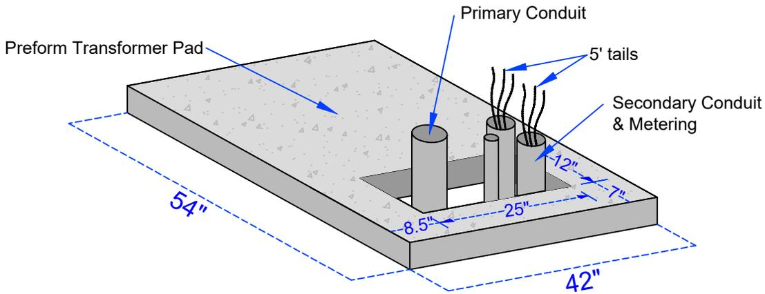
Front of Transformer **12' min.** clearance from any obstructions
